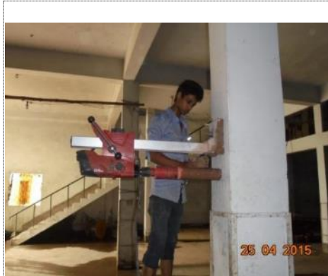
FIGURE:-DEA, CORE CUTTING OF SLAB (POWERTEX FASHION LTD, GAZIPUR)
