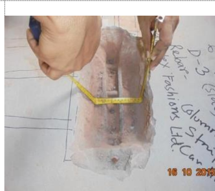
FIGURE:-DEA, CORE CUTTING OF SLAB (POWERTEX FASHION LTD, GAZIPUR)
